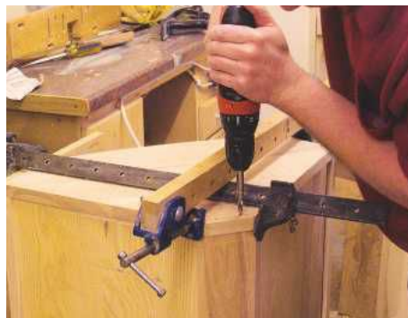
▲ Pic.15 Use Miller dowels to join the top and bottom panels to the rear upright. A special stepped drill forms the holes
